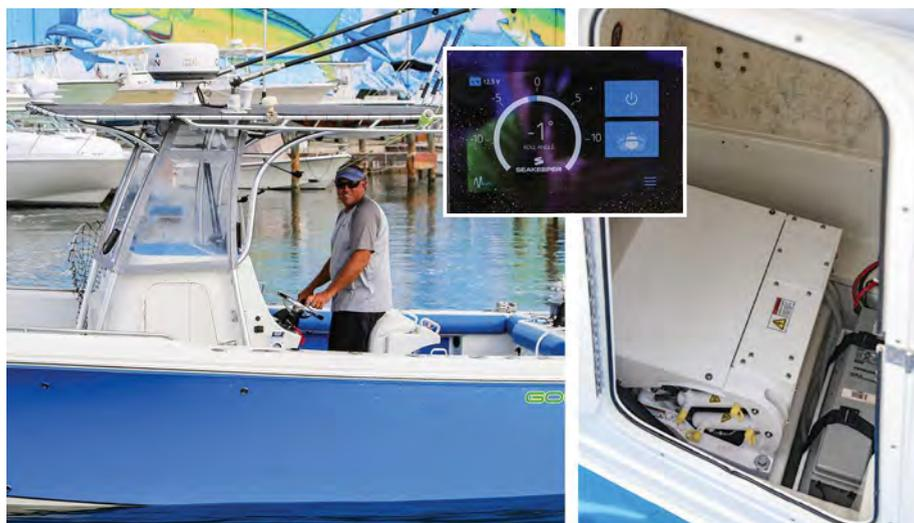
On his Sailfish 2360 (above), Capt. Ryan installed the Seakeeper 2 unit in his console (above right). Inset, touch screen panel on dash gives continuous information on the Seakeeper’s angle of roll prevention.
